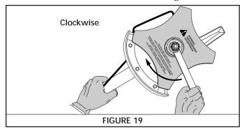
4. Remove the nut, blade retainer and blade. Store the nut and blade together for future use in a secure place. Store out of reach of children.
